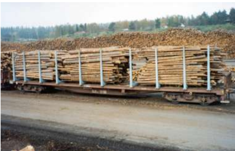
Figure 3. The wagon type used in the shuttle traffic: a typical load 50 - 55 tonne timber (max. capacity 68 tonne), no tying is needed. (Photo Teuvo Kumpare)
